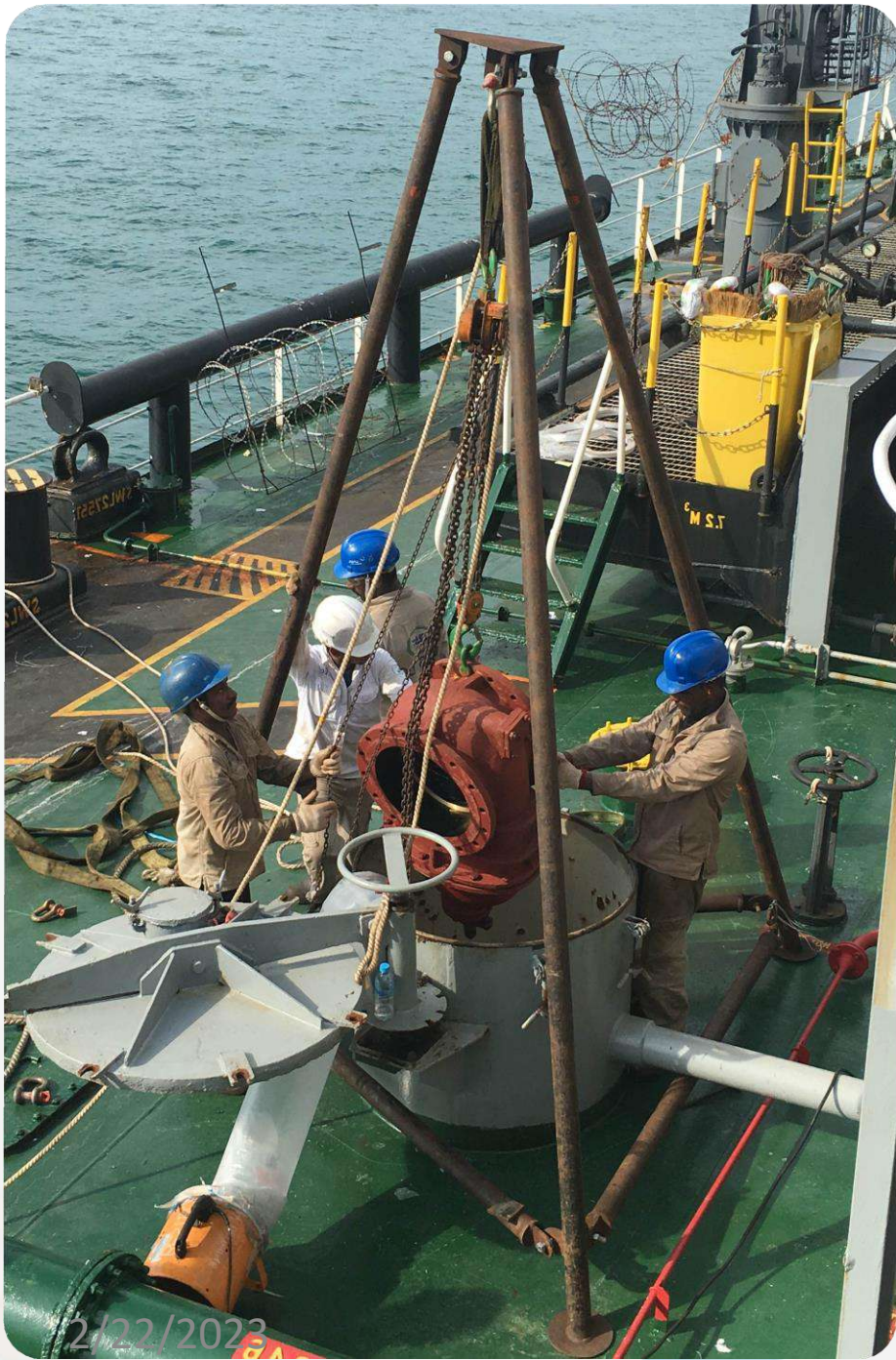
Valve removal & overhauling of PV valve , safety Valves , Butterfly & gate valve
